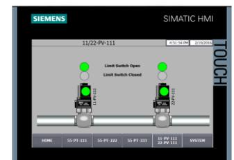
PIA Logic solver allows to indicate each individual pressure on each transmitter, whereby you can control the pipe pressure. The status of the HIPPS Valves can be shown through the limit switch boxes (positioner), which are installed on top of the actuators.
